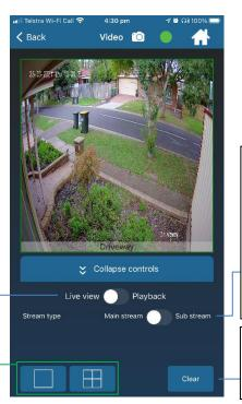
Stream Type – When a single camera is displayed, tap the toggle to switch between the Main stream and the Sub stream. Main stream offers higher quality picture and framerate but uses more bandwidth, whereas the Sub stream is lower quality but uses less bandwidth.
