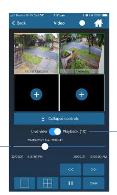
Live view / Playback – Toggles the video between live video and recorded video. When Playback is selected, this toggle also shows the current playback speed.
