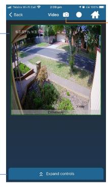
**Snapshot** – Tap to save an image of the current camera view to the camera roll. Only available with live view.
