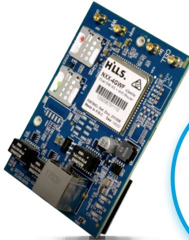
4G/WiFi Module adds 4G cellular communication capabilities to the Hills Reliance XR alarm panels, allowing alarm reporting and remote connections over the 4G mobile network via UltraSync+ Cloud.
